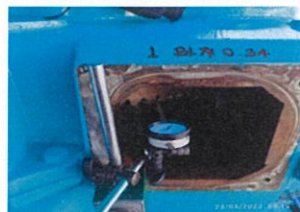
Check B/L Cell1 0.34 mm
