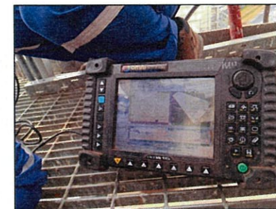
Picture No.81 : PAUT for check defects inside Desuperheater pipe
