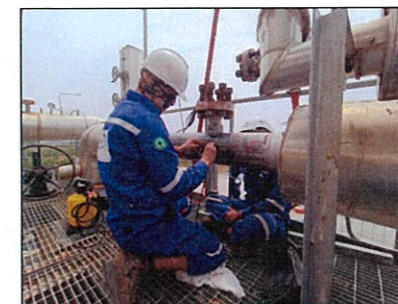
Picture No.80 : PAUT for check defects inside Desuperheater pipe
