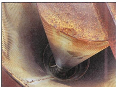
Picture No.71 : Visual inspection and remove scale on HP startup vent silencer
