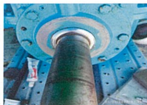
Gamma Seal Replacement
